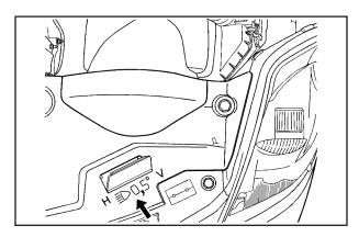
7. Locate the vertical headlamp aiming screws. They are located under the hood near each headlamp assembly. First lift the flap to access either of them. Each one is the top outboard screw by the "V" on the cover panel next to the aiming flap.
